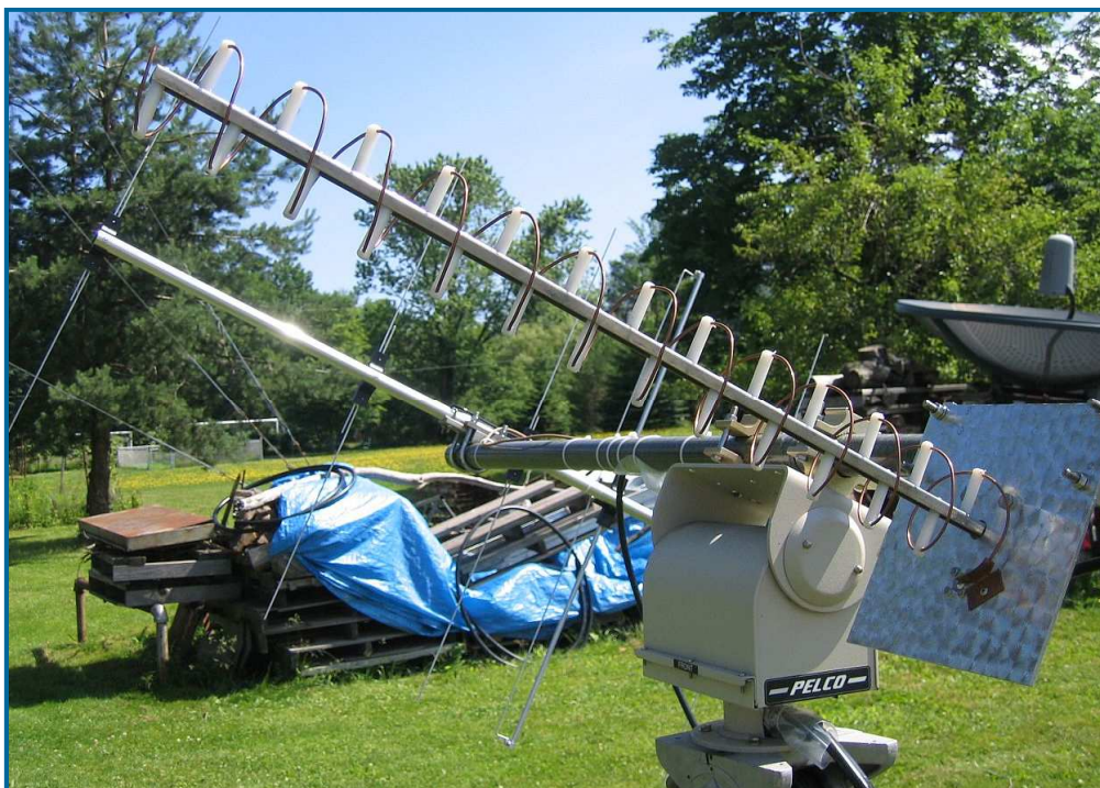
Close-up of the Home-brewed Helical Antenna
