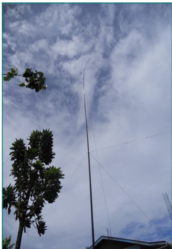
The vertical antenna for 160/80/40m bands
